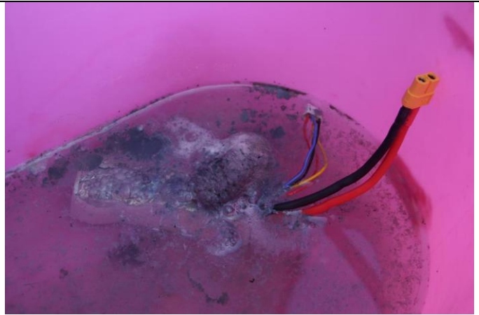
How to properly dispose of LiPos. Put them in salt water and stand back. (Pink bucket optional) This was in the shark
