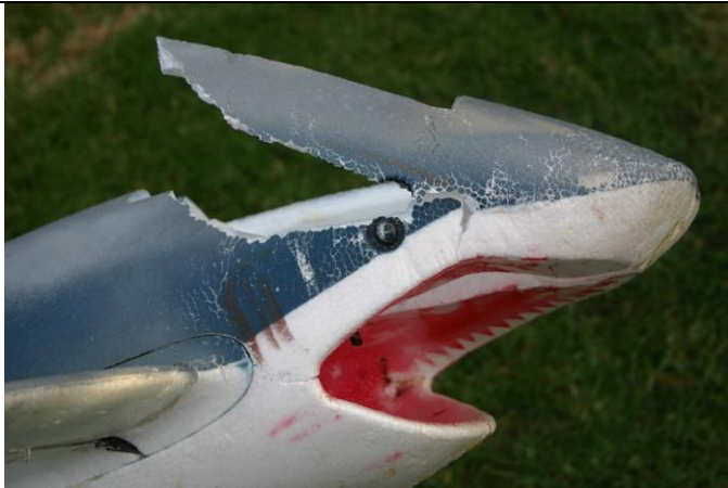
Wayne Drinkwater's Shark after it threw turbine blades through the controls at openday.
